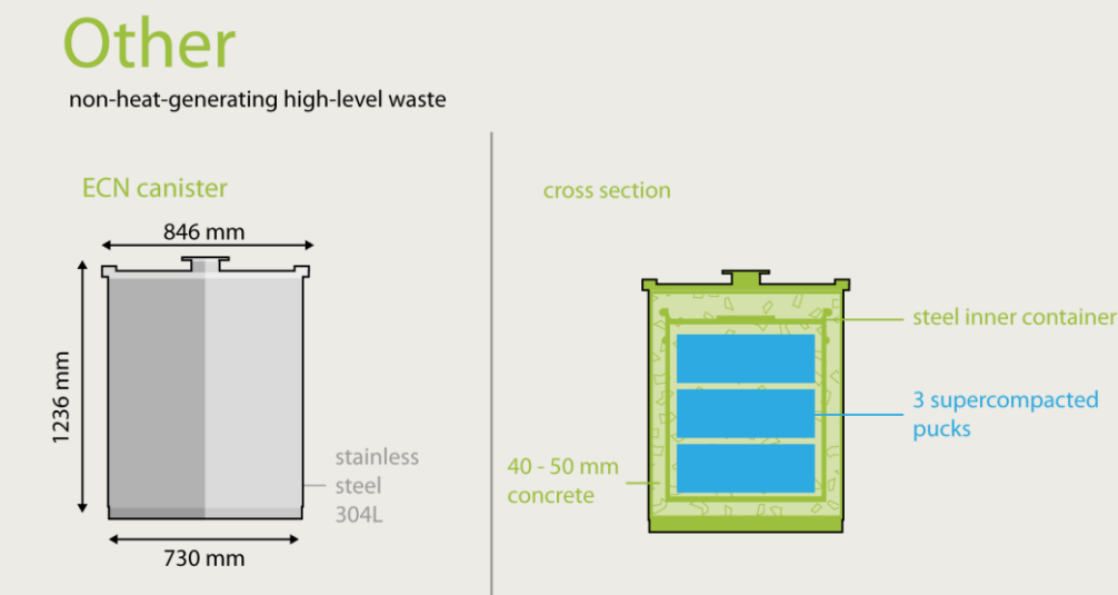
Figure 4-3. Schematics of ECN canister with (super)compacted pucks; dimensions in mm.
