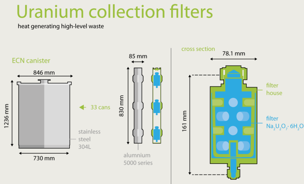
Figure 3-5. Schematics of Uranium collection filter and ECN container; dimensions in millimetres [NRG, 2009].
