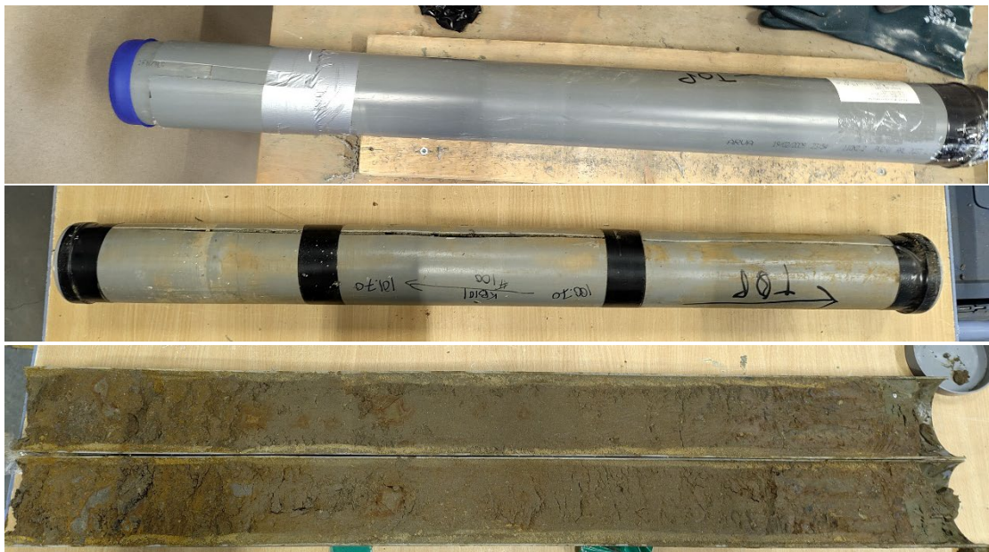
Figure 3.1: Example of a sediment core as received. Top: outer liner. Middle: original liner that had already been opened in the past. Bottom: Reopened liner with brown colour as a clear sign of oxidation.
