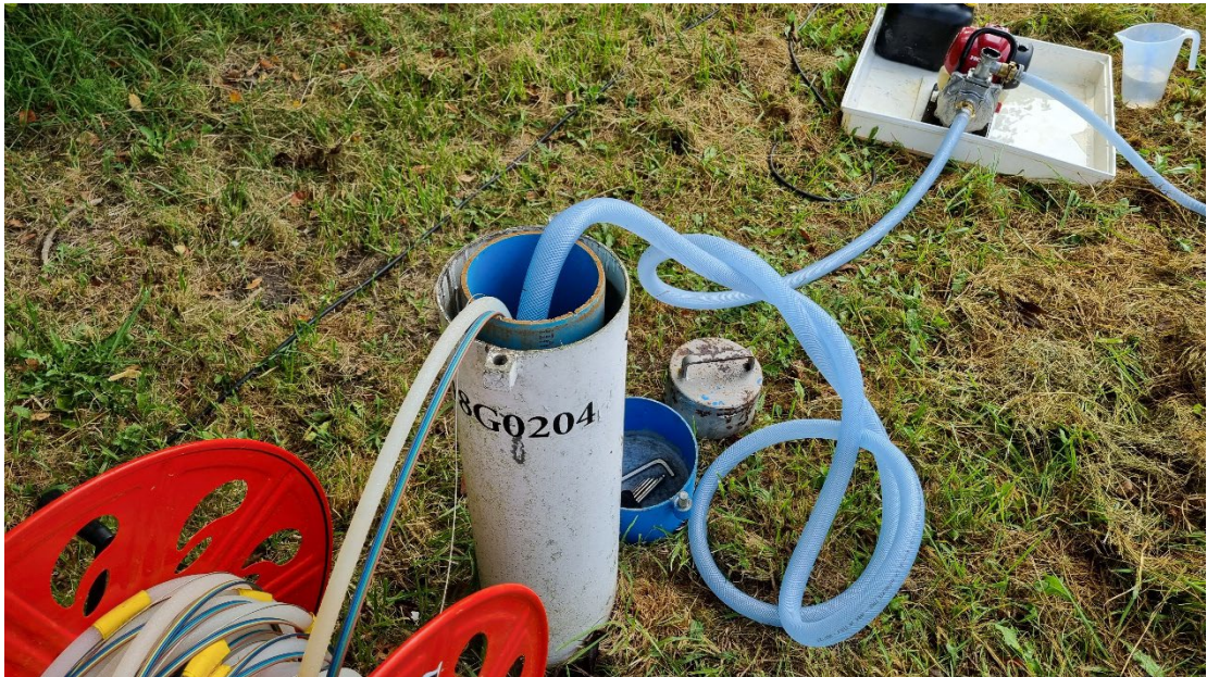
Figure 3.4: Well B48G0204 (Overzande), with a large well diameter of 15 cm.
