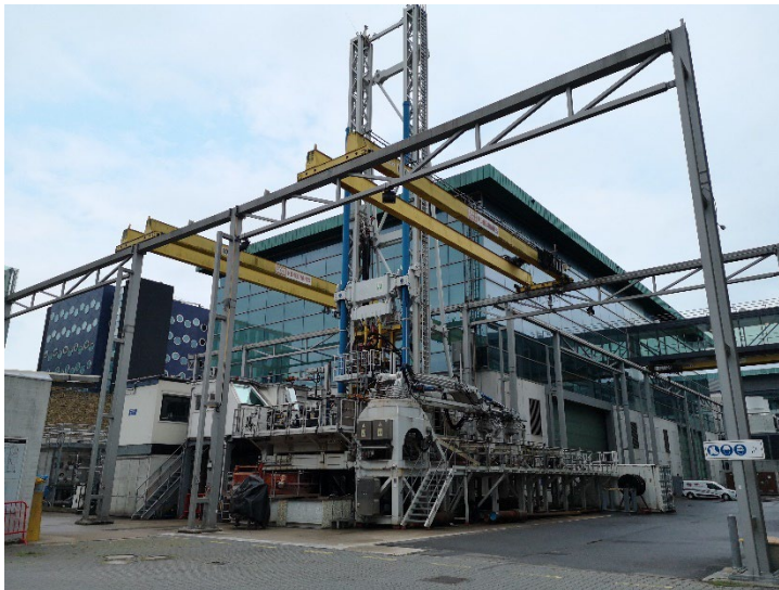
Figure 20: Full operational drill rig with 2 research wells 450 meters deep at Rijswijk Centre for Sustainable Geo-energy
