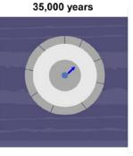
At this point, it is assumed that all the overpacks fail and the total including glass surface area. fractures in the vitrified waste form, becomes available for dissolution. The dissolution rate radionuclides is determined by the cracking factor and the alteration rate of class
