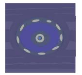
The waste has cooled down and no longer heats the clay host rock. Reactions between cement minerals and dissolved species in the incoming clay pore water have led to a reduction in pH in the vicinity of the overpack. The anoxic corrosion rate of the overpack has increased. The vitrified waste form has not come into contact with water.
