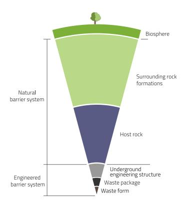
The relative contributions to safety of the various barriers at different times after closure of a disposal facility and the ways that they interact with each other depend upon the design of the disposal system. The design itself is dependent on the geological environment in which the facility is constructed. Consequently, the multibarrier system can function in different ways at different times in different disposal concepts.
