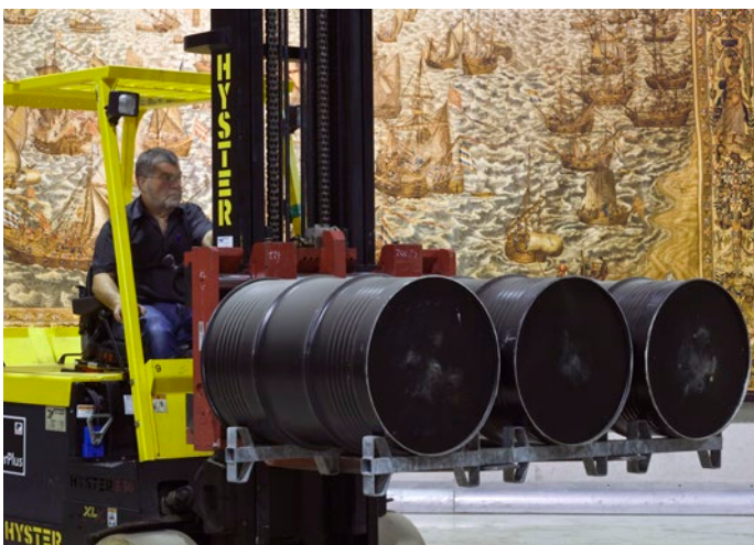
Forklift trucks for emplacement of three 200 l drums of one 1000 l concrete container
