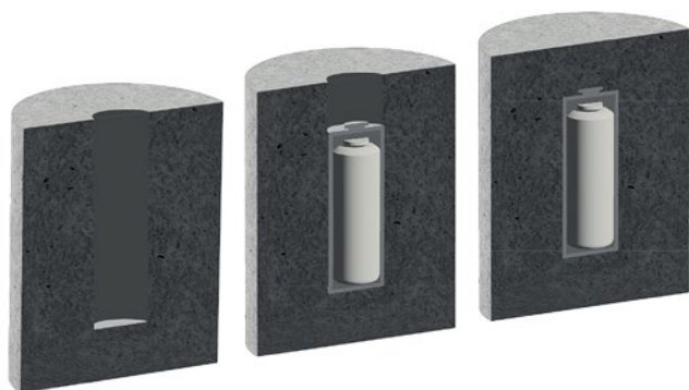
Figure 4-10: Encapsulation of vHLW in supercontainers.
