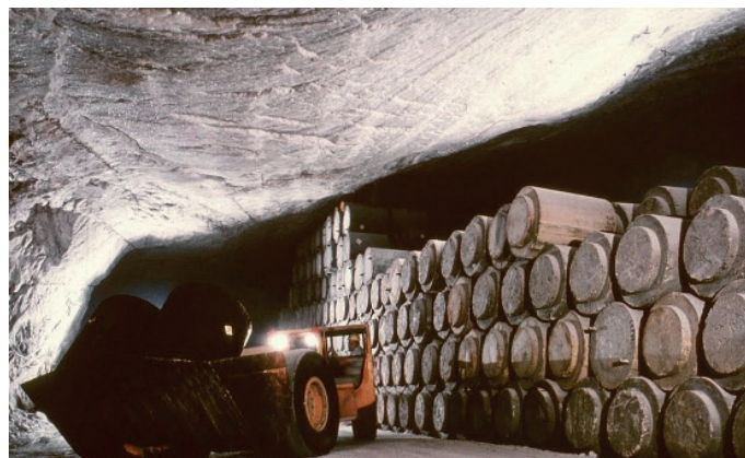
Figure 2.6) Drums with concrete shielding emplaced within the Asse II mine. Photo: Bundesgesellschaft für Endlagerung mbH.
