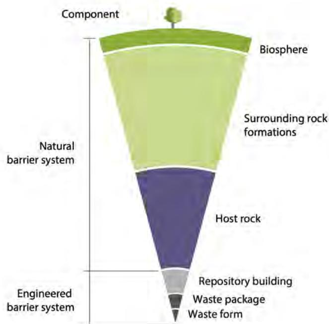
Figure 1: Components of a geological disposal system with two main barrier systems, engineered and natural burial systems [6].
